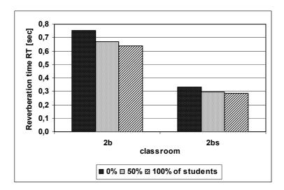
**Fig. 5.2** Room acoustic balance for the Baumberge Schule; average reverberation times measured in empty, half-full and fully-occupied room
