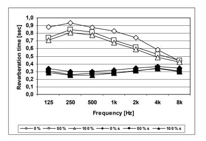
**Fig. 5.5** Frequency-dependent reverberation time of the classroom in the Baumberge Schule before (□) and after (■) the refurbishment when empty, half-full and fully occupied
