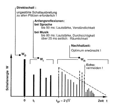
Fig. 2.4Schematic room impulse response. Illustration taken from FASOLD AND<br/>VERES, P.149.<br/>ti: Time between direct sound and early reflection in ms<br/>tgr: Time limit for the transfer of early reflections to diffuse reflections<br/>(reverberation) in ms<br/>V: Volume in m³
