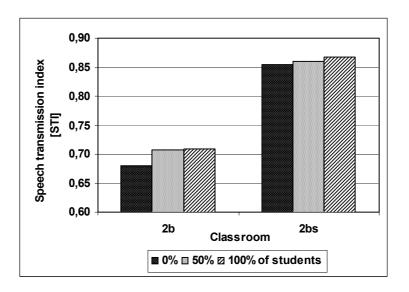
**Fig. 5.13** Speech Transmission Index STI in the classroom at the Baumberge Schule before (2b) and after (2bs) the refurbishment, measured in the empty, half-full and fully-occupied room
